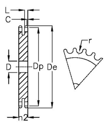
C = 4 D = 30 De = 541 Dp = 525.84 For chain size = 1  $1/4 \times 3/4$ For chain type = 20 B-2 b2 = 54.6
